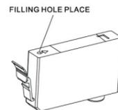
1. Seal the outlet with sealing tape and place the cartridge on paper towel or other absorbent material in case of excess ink. Make sure the outlet is facing down.
